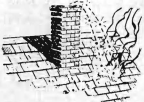
Sparks on combustible roofs
